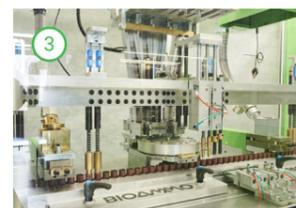
**Equipped with servomotors, which allow the customization of the vibration of both dispensers.**
